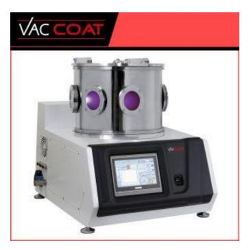
PLD – T is a high vacuum thin film deposition system enables to deposit different materials by both Pulsed Laser Deposition and so thermal evaporation technique. It can deposit complex materials and crystalline structures onto substrates with very little setup involved.
